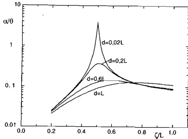
Figure 2. Isoplanatic angle dependence on the corrector location.
