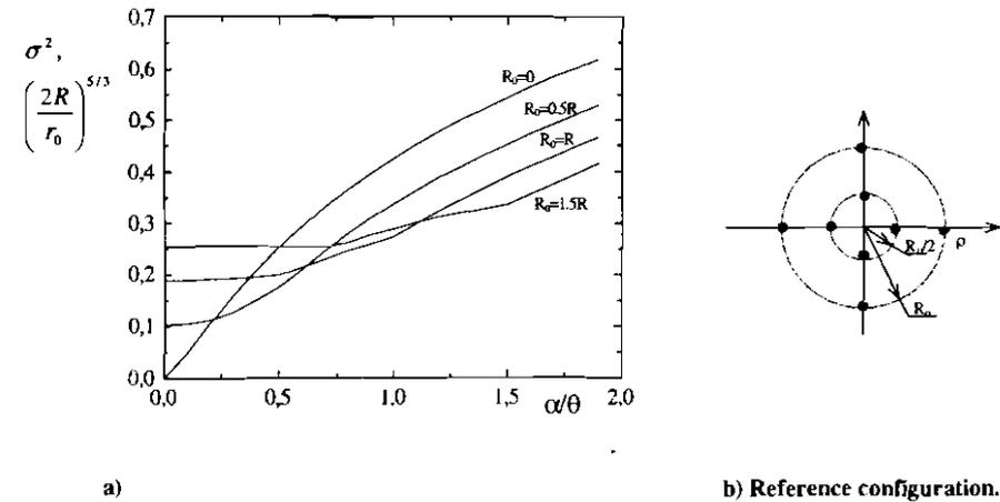
Figure 4. Mean square error in a multireference adaptive system.  $R_0 = R\alpha/\theta$ .
