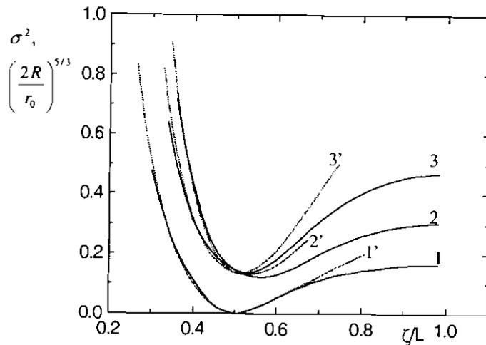
Figure 3. Mean square error dependence on the phase corrector location. 1 - one thin layer,  $y=0.5L$ ; 2 - two layers,  $y_1=0.4L$ ,  $y_2=0.6L$ , 3 - three layers,  $y_1=0.4L$ ,  $y_2=0.5L$ ,  $y_3=0.6L$ . 1', 2', 3' - piston not removed.
