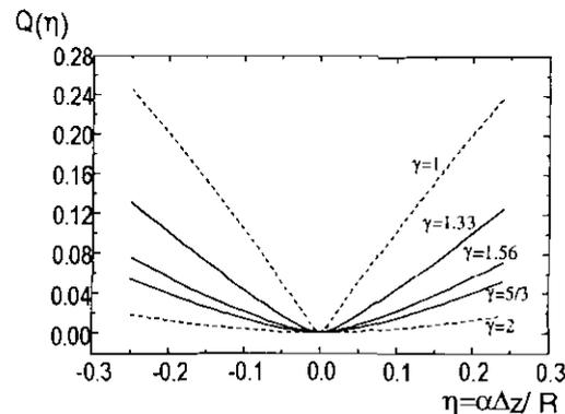
Figure 6. The mean square aberration suppression factor.
