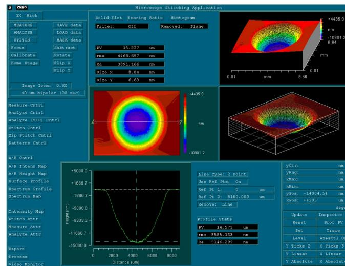
Fig.1 Output of Zigo interferometer for Microscan-2000
